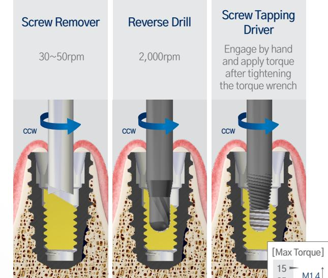
※ Most screws can be removed using 4 types of tools by diameter.
